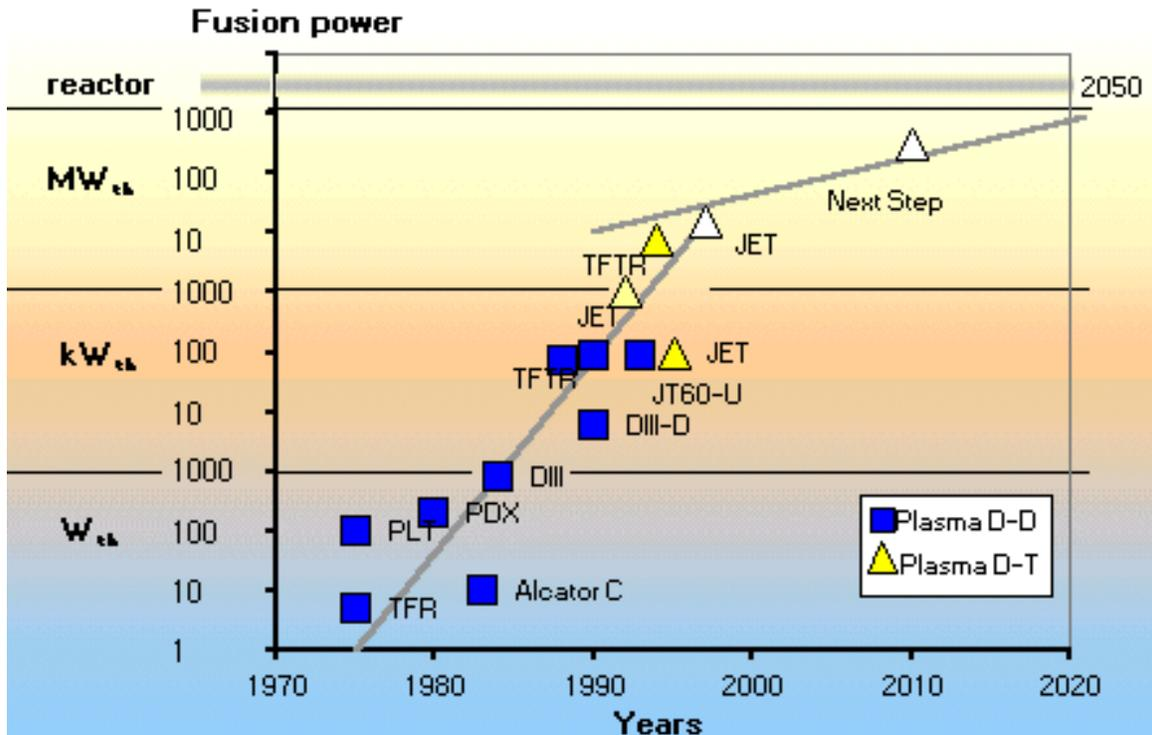
Figure 28. The path towards fusion power production.
