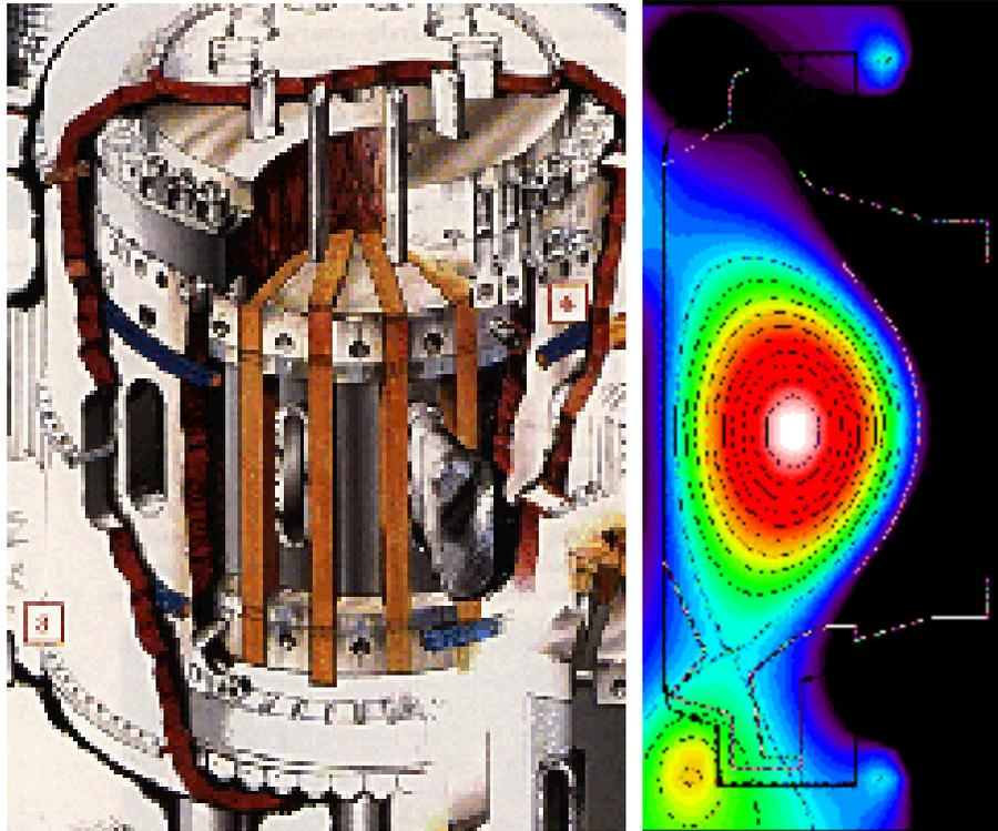
Figure 15. ALCATOR, MIT Tokamak plasma shape showing the divertor at the bottom left.
