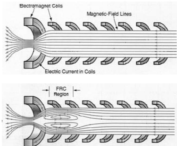
Figure 1. A basic configuration linear mirror (Top) and a mirror with a Field Reversed Configuration (FRC) end plug.
