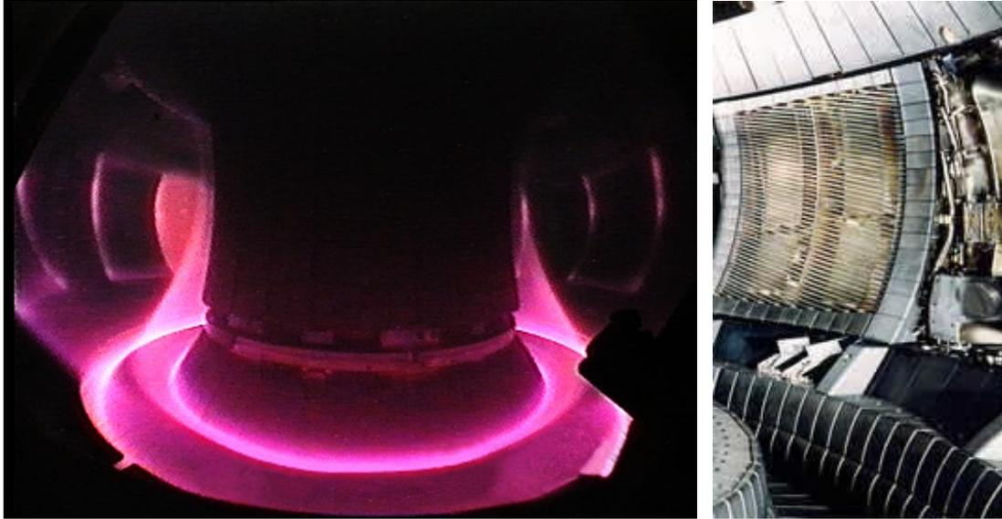
Figure 16. Asdex-U plasma and divertor plates inside reactor vessel at the Max-Planck Institut, Germany.
