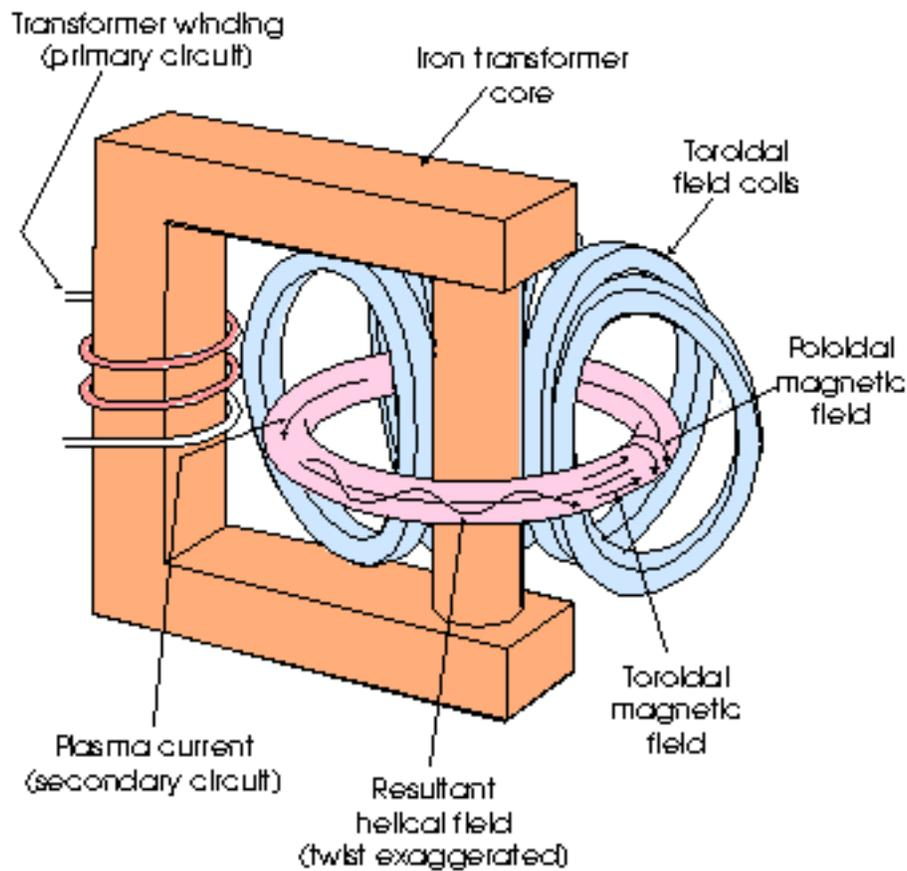
Figure 5. Tokamak concept showing the transformer core, toroidal field coils and toroidal magnetic field, poloidal magnetic field and the resultant helical field.
