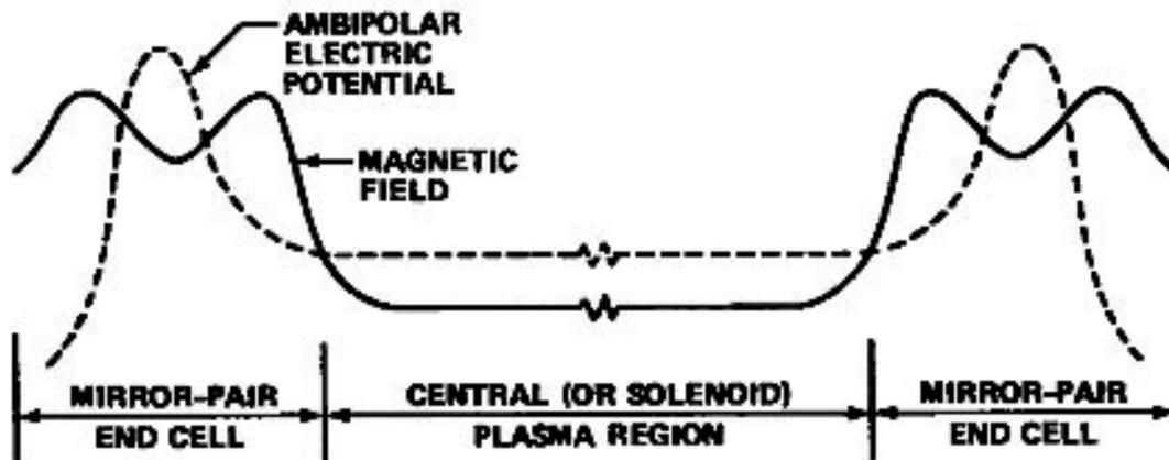
Figure 2. The Tandem Mirror fusion concept, showing the Ambipolar Electrical Potential. A mirror pair end cell is located at each end of a uniform central solenoid field.
