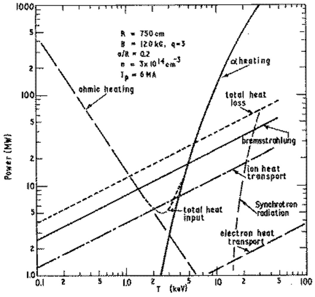
Figure 26. Energy balances in a typical Tokamak.
