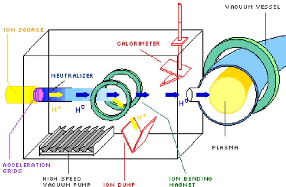
Figure 14. Neutral particle beam heating of a plasma.
